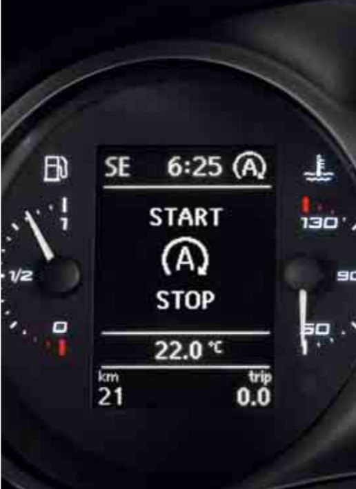
The Start/Stop System can be turned on or off at the push of a button. An illuminated symbol tells you when it's been activated.
