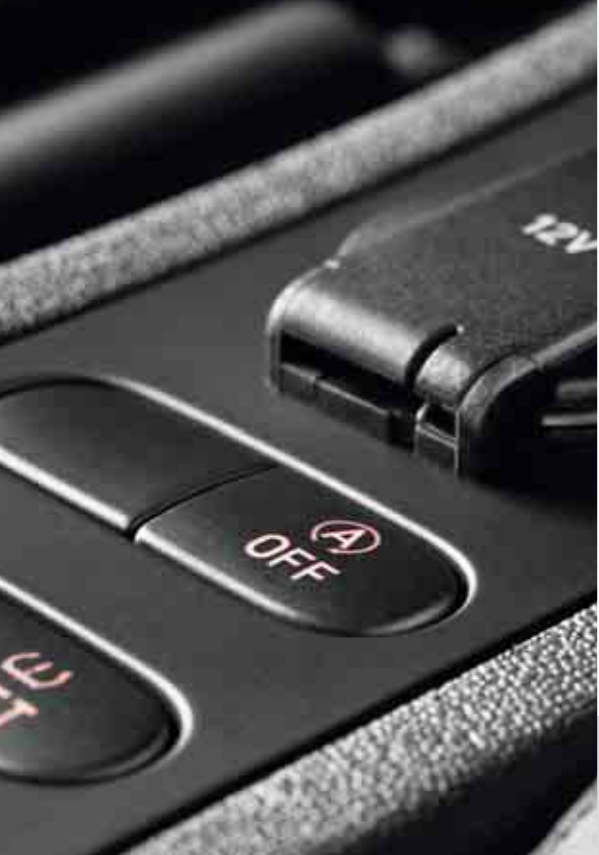
The Start/Stop System can be turned on or off at the push of a button. An illuminated symbol tells you when it's been activated.
